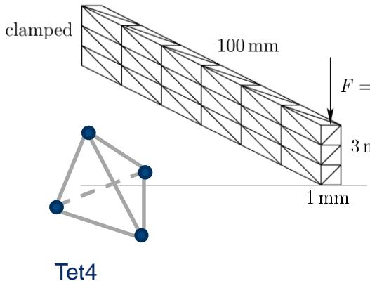
$$\begin{aligned}E &= 2.07 \cdot 10^{11} \text{ N/m}^2 \\ \rho &= 7850 \text{ kg/m}^3 \\ \nu &= 0.0 \\ n_x &= 50 \\ n_y &= 1 \\ n_z &= 3 \\ F &= 2 \text{ N} \\ t_{\text{end}} &= 20 \text{ ms}\end{aligned}$$
